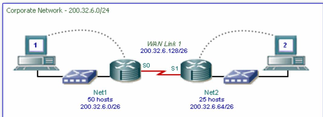
A corporate network has two networks linked together via a single WAN link. The network address of 200.32.6.0/24 has been divided into four equally sized subnets. The subnets design is as follows:-
